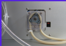
Peristaltic pump automated to keep dip tank at set level
