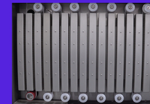
Drying chamber variable material path 3 m to 12.5 m
