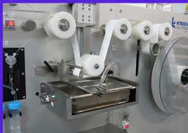
Optional dip tank with peristaltic pump and fluid level sensing
